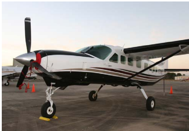
Cessna Grand Caravan - Equipped with Leica RC-30 camera, IMU & OPTECH 3100 LIDAR Unit
